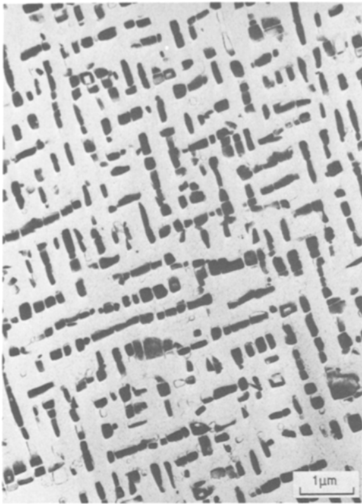
Figure 4 Aligned rows of cubic \gamma' particles in Ni 22–13 after ageing for 239 h at 1073 K.
