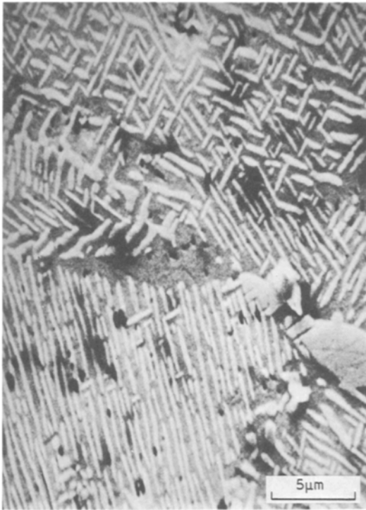
Figure 7 Plates of \gamma' formed in Ni 37–12 after ageing for 698 h at 1073 K.
